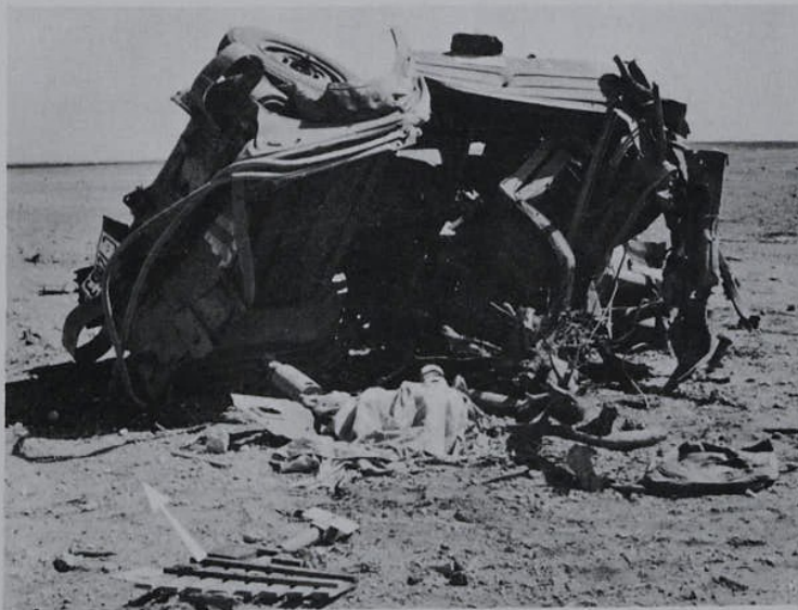
FIGURE 13. ROUND 3. CHAMP AT 1860 ft. NOTE LOWER HALF OF DUMMY DRIVER IN WRECKAGE
